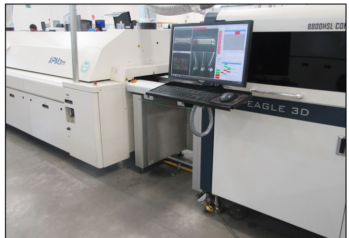
A 3D automated optical inspection unit has been installed following reflow on each SMT line.
