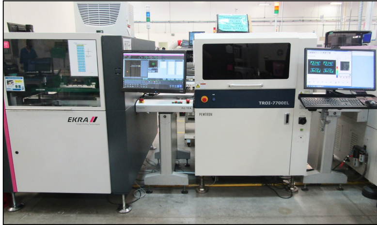
A 3D solder paste inspection (SPI) unit is installed behind each SMT line's screen printer.
