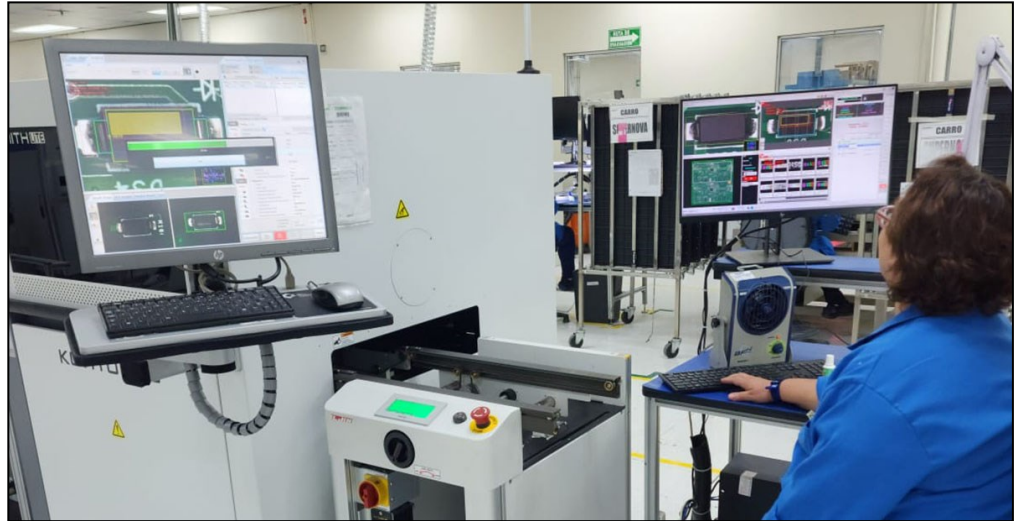
Automated optical inspection (AOI) is critical to monitoring the the pin-in-paste process.
